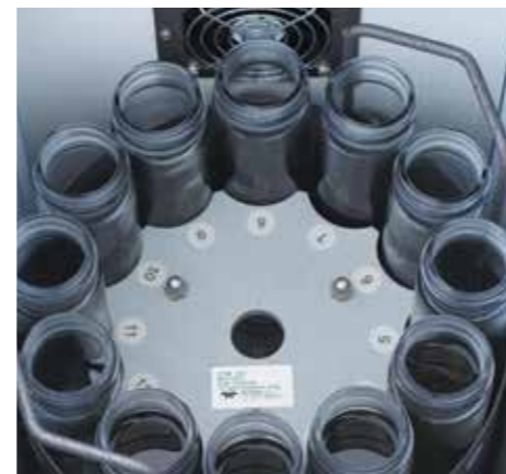
Water sample carousel in refrigerated autosampler
