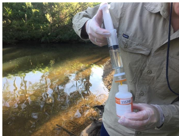
Figure 4 Example of pouring from the D bottle into the syringe (left); and filtering the sample into a DES dissolved nutrients bottle using a pre-filter (right)
