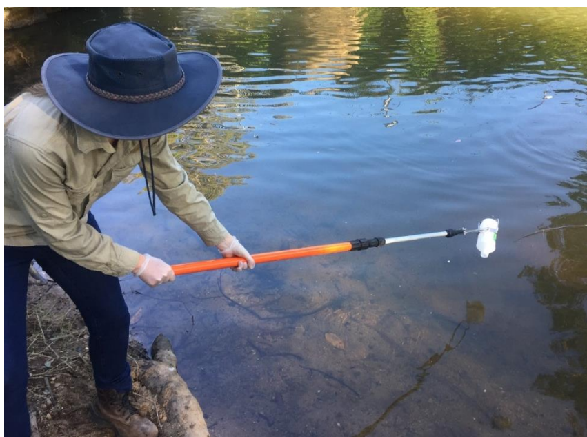
Figure 3 Sampling pole with the total suspended solids bottle inverted in preparation to collect a water sample
