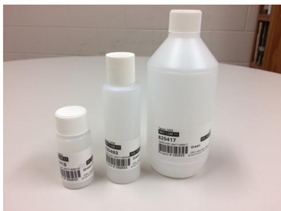
Figure 1 Sample bottles for dissolved nutrients, total nutrients and total suspended solids (left-right)
