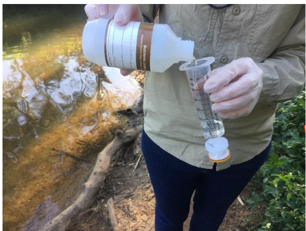
Figure 4 Example of pouring from the D bottle into the syringe (left); and filtering the sample into a DES dissolved nutrients bottle using a pre-filter (right)
