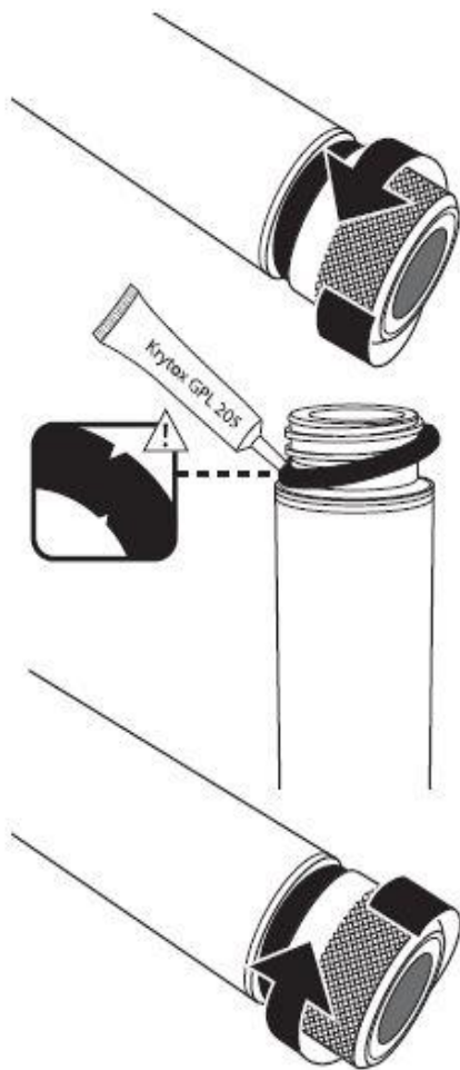
Figure 66 ProDSS ODO cap replacement
