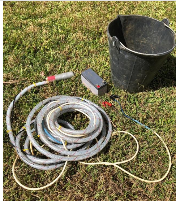
Figure 2 Rule IL280P slimline submersible pump with connection to 12V battery and purging bucket
