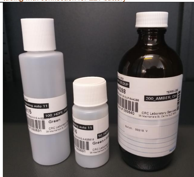
Figure 3 Bottles for collection of unfiltered and filtered nutrients and pesticide samples (left to right)
