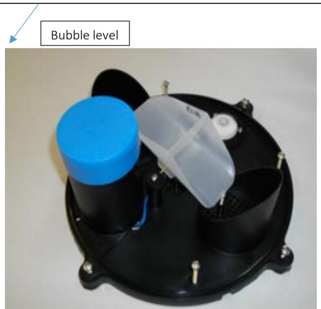
Figure 4 RainWise tipper bucket rain gauge internals
