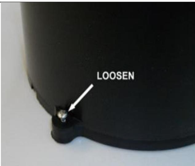
Figure 3 RainWise funnel fastening screws
