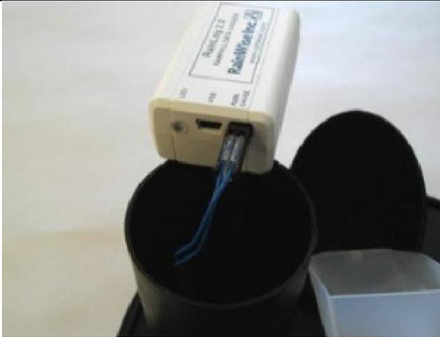
**Figure 5** RainLog 2.0 data logger connector
