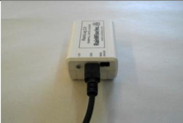
Figure 1 RainLog 2.0 logger with data transfer cable
