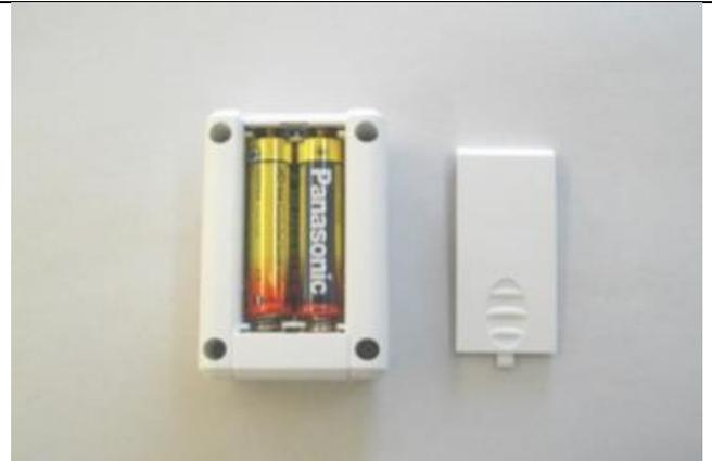
Figure 1 RainLog 2.0 battery installation
