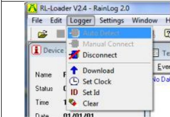
**Figure 8** RainLog clear data, set name and clock functions. **These three items MUST be completed prior to deployment.**
