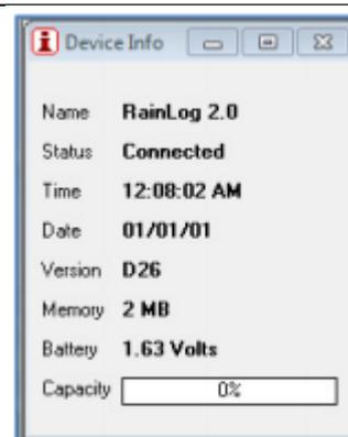
**Figure 9** RainLog 2.0 logger data. Ensure battery and memory capacity is sufficient before deployment.
